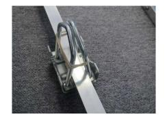
Take the flexible Reflector Element (longest), undo the nut holding the bolt on the plastic fitting. Holding the boom, with the labels up, push the element assembly onto the boom pushing the bolt through the hole (furthest away from the end of the boom). Screw the nut back on the bolt coming through the hole and tighten (slightly more than finger tight), fixing the element in place.
