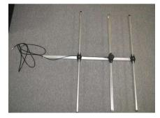
The Antenna should be fixed to the mast using the clamp provided (mounted behind the reflector element) in either a horizontal (common mounting) or vertical stance to best suit your study environment. Do check with a hand-held Yagi which polarisation is best suited.
